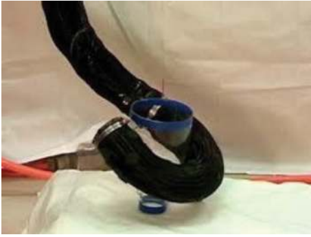
FIGURE 1: A continuum robot grasping and manipulating a fragile (glass) object, using its compliant backbone to adapt to the object's shape.
