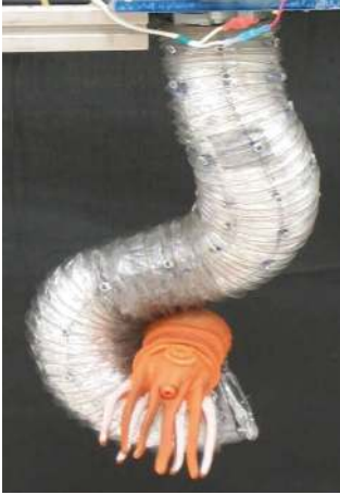
FIGURE 3: Air-Octor Continuum robot. This two-section, six-degree-of-freedom robot bends a pneumatically inflated core tube using six tendons.
