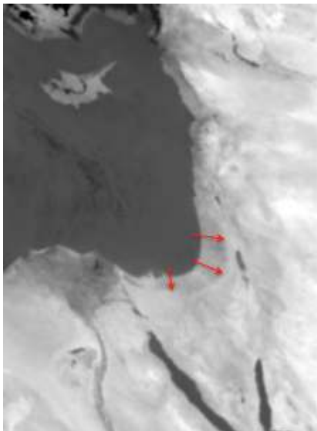
Fig. 4. MSG channel 9 ( 10.8\ \mu\text{m} ) brightness temperature from 7 July 2010 14:00 LT. The three red arrows point to the thermal impact of the SB on the surface temperature. An animation depicting the progression of the SB from 09:30 to 17:00 LT can be found in the supplementary.
