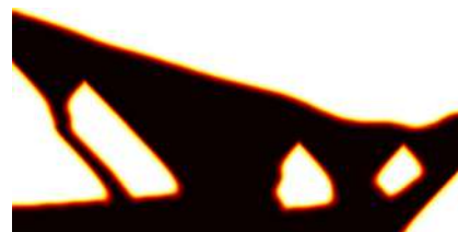
Fig. 16 Design obtained with overhang filter using a conventional initial design. To obtain good results, starting with a fully solid design is recommended. C = 1.69C_{\text{ref}}
