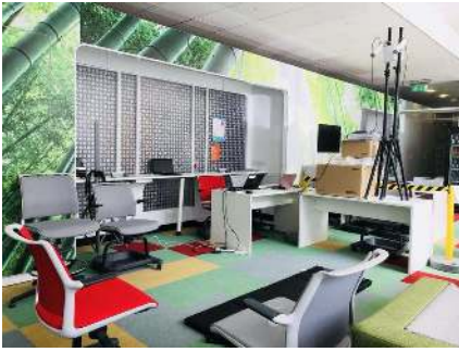
Fig. 1. Environment of the experimental setup with radar antennas mounted on tripods and sources of static clutter (furniture) shown.
