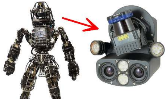
Fig. 2. The Atlas robot’s primary sensing is provided by the Carnegie Robotics Multisense SL sensor head which is equipped with a stereo camera and a rotating LIDAR scanner. In this work we use only the stereo camera, except in Sect. IV-A where we compare the terrain estimated by the stereo camera to that estimated using the LIDAR. (photo credits: Boston Dynamics and Carnegie Robotics)
