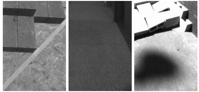
Fig. 7. Texture in industrial and office environments such as the brick, wood (DRC Trials, left) and carpet (center) is sufficient to produce accurate terrain reconstructions, however the poor gain control in an example from the DRC Finals (right) cannot produce a reliable reconstruction.
