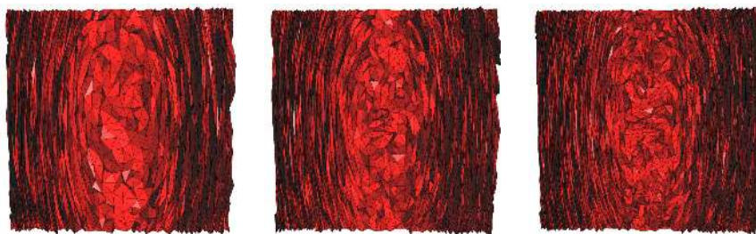
FIG. 1.8. From left to right, views (cut through the plane y = 0 ) of the unit meshes \{\mathcal{H}_{4,\alpha}\}_\alpha with respect to \{\mathbf{M}_4(\alpha)\}_\alpha for a complexity of 4000, 8000 and 16000.
