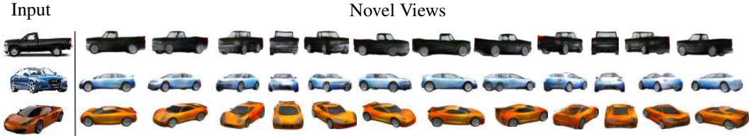
Figure 6: Qualitative results of novel view synthesis on real data. Our model generates high quality views of previously unseen data. We use the model trained on ShapeNet and evaluate on the Cars [19] without retraining.
