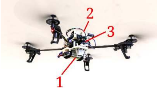
Fig. 7: Experimental platform with (1) down-looking camera, (2) on-board computer, and (3) inertial measurement unit.
