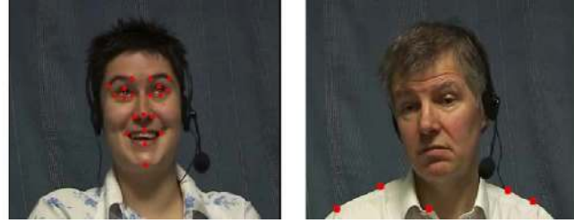
Fig. 2. Illustration of tracked points of (left) the face ( T_{f1} - T_{f20} ) and (right) the shoulders ( T_{s1} - T_{s5} ).
