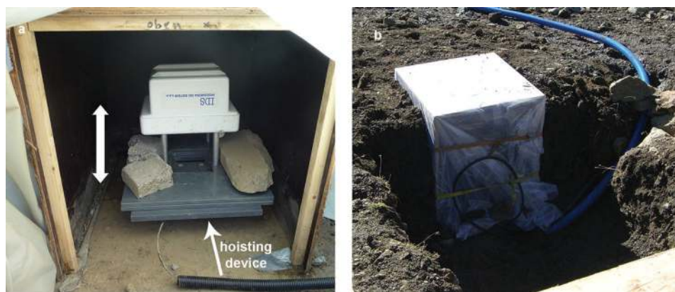
Fig. 1. Assembling of radar set-up. (a) The antenna is lifted and lowered by a hoisting device during measurements. (b) The arrangement is located in a wooden box buried in the ground.
