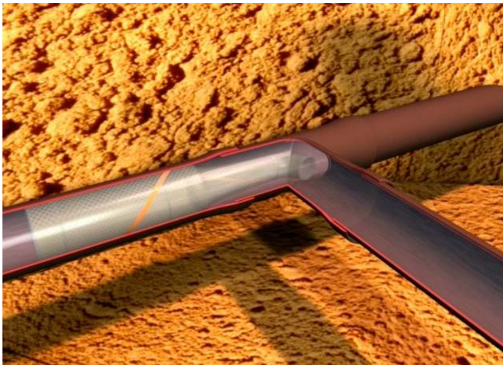
Figure 46: A pipe crawling robot navigating a corner. Such an arrangement resembles a “Feynman Sprinkler,” and it is not immediately clear what forces would affect the head of the robot.
