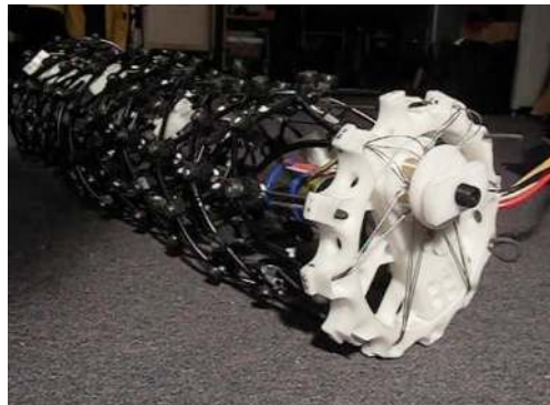
Figure 18: A still taken from high-speed video of the final worm cam mechanism. There is slack in the top four cable pairs, but the cam head prevents them from tangling.
