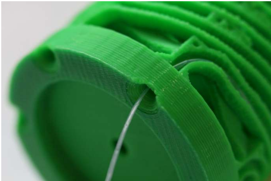
Figure 44: A first prototype of a printed wormlike robot that is 4 cm in diameter. The entire device is shown on top, while a detail of the unfinished cam mechanism is shown on bottom. Fishing wire is used as an actuation cable, which sits inside a thin Teflon tube, which in turns rests inside a groove in the ABS plastic. It can also be seen running through small guide holes inside the robot (top) to make a hoop actuator. At this scale, the texture of the printing would likely cause problems for the cables.
