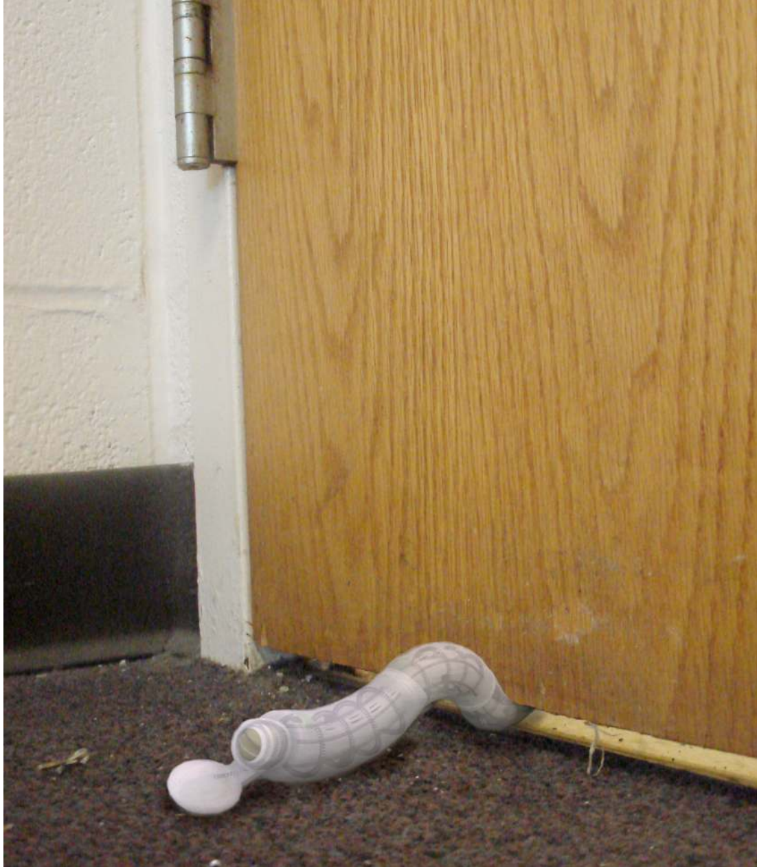
Figure 2: A computer rendering I made of an early concept for the DARPA ChemBot project. Two and a half segments are shown squeezing under a door. The pad at the front has directional spikes for inchworm-like attachment and locomotion. An apparatus at the front is based on the aplysia mouth and could take small samples from the environment.
