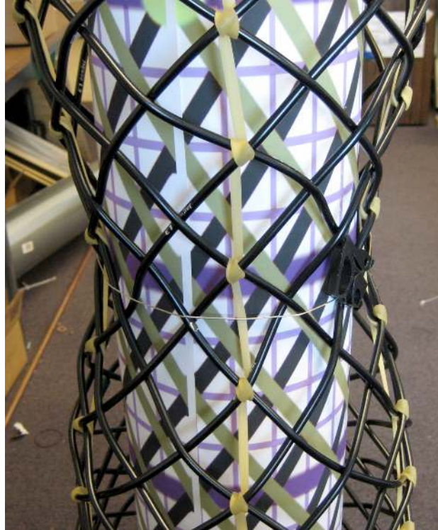
Figure 12: The first prototype keeps its anisotropic strain properties by weaving bicycle brake cable sheathing and securing it with latex tubing that also acts as a return spring. This method of construction did not keep the mesh in good alignment after several trials. In this figure, a single hoop actuator has been installed and is in the constricted position.
