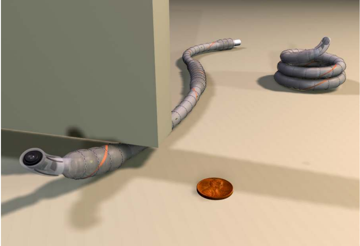
Figure 3: Final concept robot design for the DARPA ChemBot grant. The robot could roll up into a ball, and squeeze under a door frame. Unlike our first design, the peristaltic waves would move smoothly down the body.
