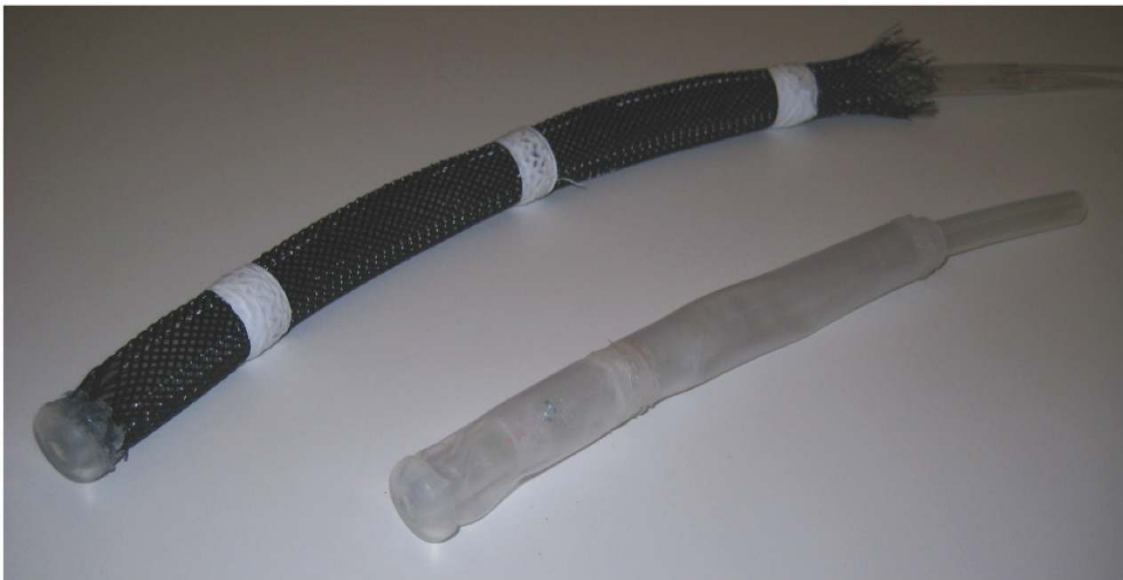
Figure 5: (Left) A previous worm-like robot with discrete actuators surrounded by a braided mesh. (Right) The inner actuator core that inflates the mesh [Mangan, et al. 2002].
