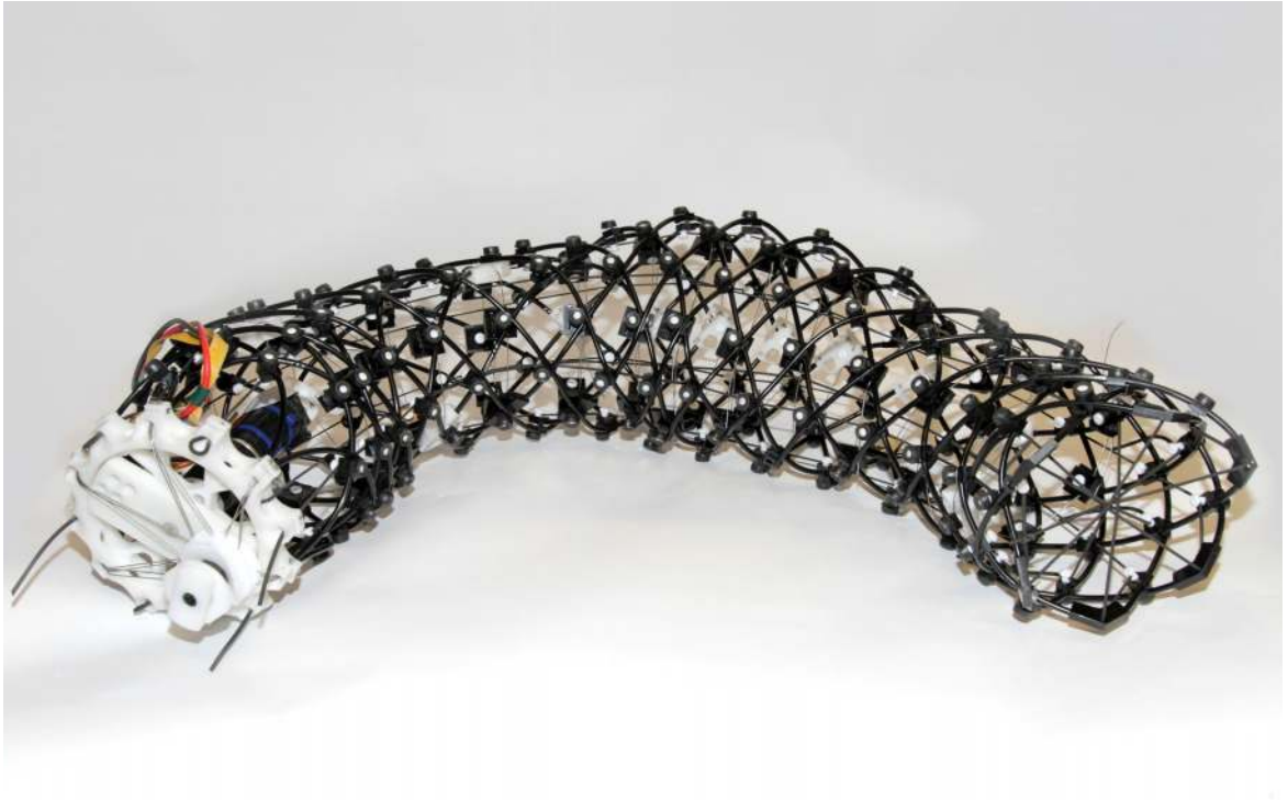
Figure 1: A robot that creates peristaltic motion with a continuously deformable exterior surface.
