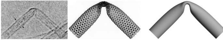
Figure 1. Buckling at the nanoscale: experimental observation, atomistic calculation (Reprinted with permission from Iijima, S., C. Brabec, A. Maiti, and J. Bernholc: 1996, Structural flexibility of carbon nanotubes. Journal of Chemical Physics 104 (5), 2089-2092. Copyright 1996, American Institute of Physics.) and exponential Cauchy-Born rule-based continuum calculation
