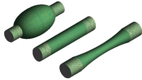
Figure 4: McKibben air muscle actuators.
