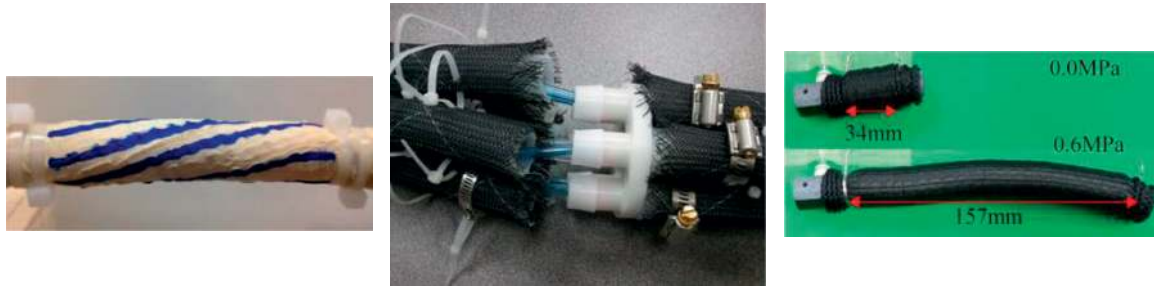
FIGURE 8: Pneumatic artificial muscle—fiber material and braided structure [206–209].
