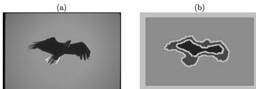
Figure 3. Demonstration of the “contour-as-a-texture” problem using a real image. (a) Original image of a bald eagle. (b) The groups found by an EM-based algorithm (Belongie et al., 1998).
