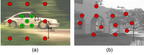
Figure 3: For each training image, N_E example centroids are used. The positions of positive examples are shown with pluses, and negative examples are shown with minuses. In (a) a class image generates examples relative to the known centroid, to encourage localisation in the classification map. In (b) a background image generates negative examples at false detections of K_1 , so clutter can be explicitly trained against.
