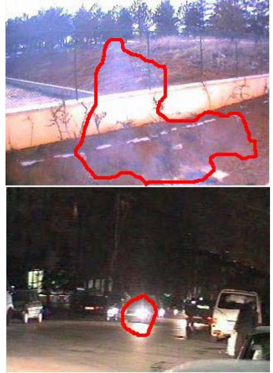
Fig. 4. Two moving objects in video: smoke image (top), and a vehicle (bottom). The object boundaries are determined by the background subtraction algorithm.
