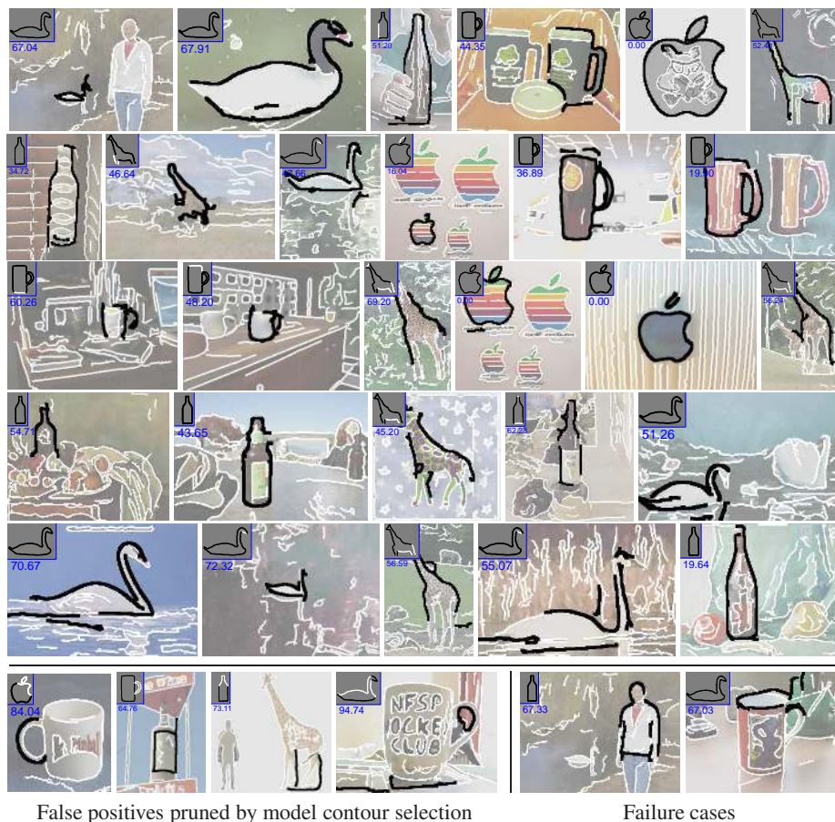
Fig. 6. Examples of contour context selection on model and image contours in ETHZ Shape Classes. The first five rows show detected objects from image with significant background clutter. In the last row, the first four cases are false positives successfully pruned by our algorithm due to bad configurations of selected model contours. The last two are failure cases. Each image only displays one detected object instance.
