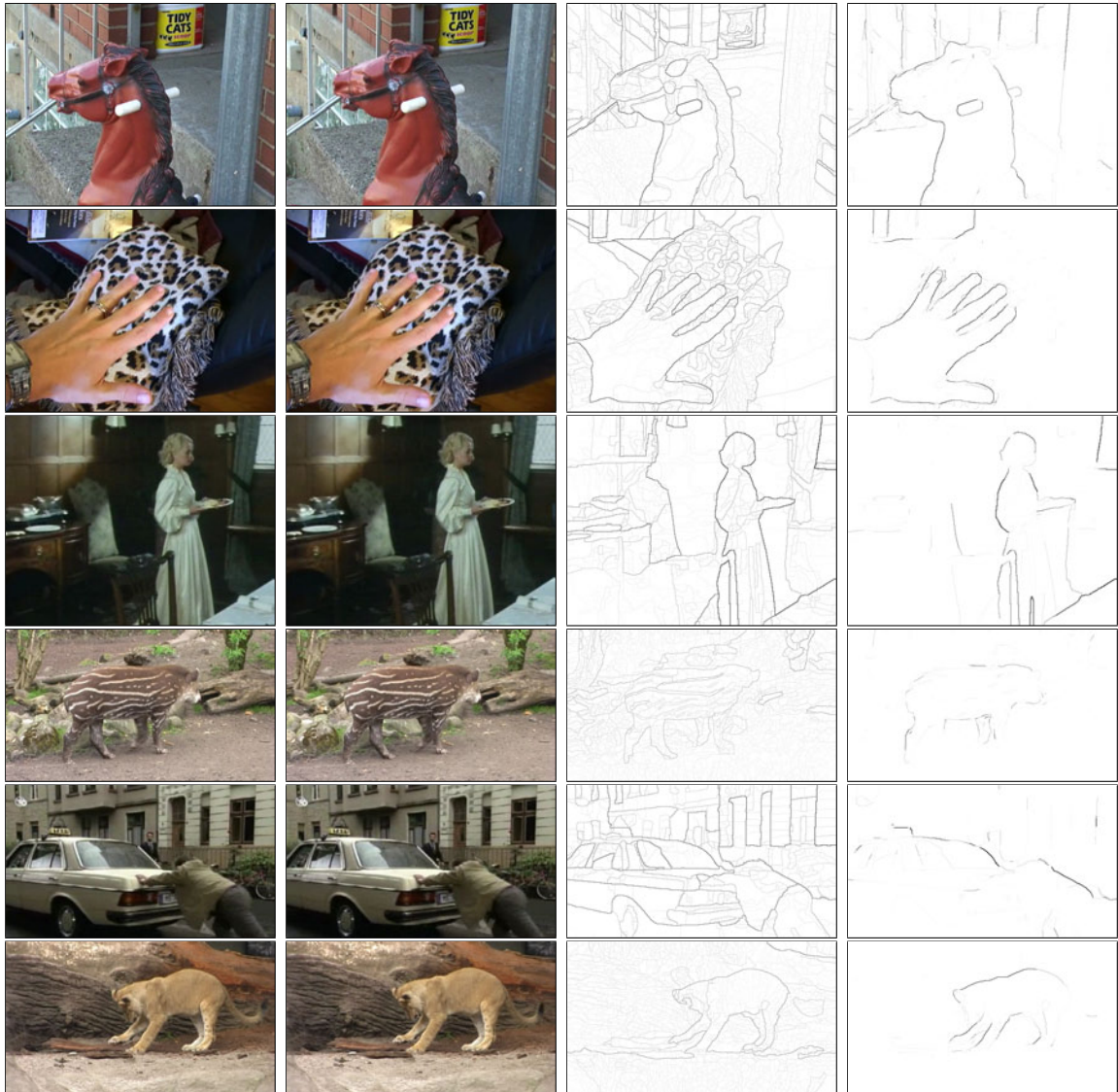
Figure 4.4: Occlusion boundary detection results. From left to right: Two consecutive video frames, Ultrametric Contour Map for the first frame created from the gPb+mg contour detector, and boundaries reweighted according to our occlusion classifier.
