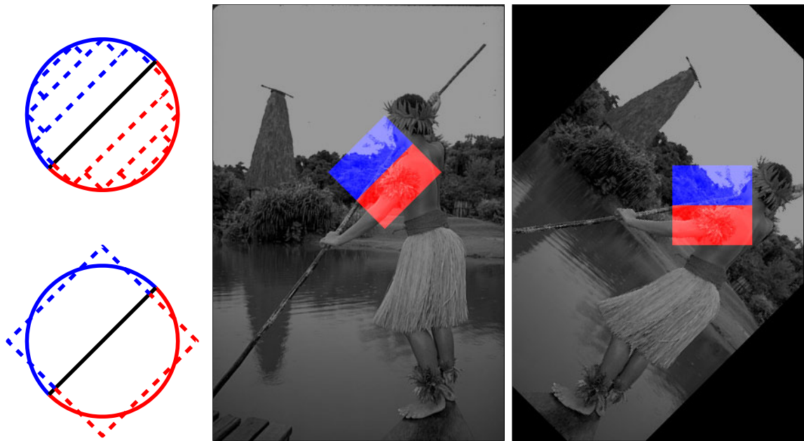
Figure 2.6: Efficient computation of the oriented gradient of histograms. Left: The two half-discs of interest can be approximated arbitrarily well by a series of rectangular boxes. We found a single box of equal area to the half-disc to be a sufficient approximation. Middle: Replacing the circular disc of Figure 2.3 with the approximation reduces the problem to computing the histograms within rectangular regions. Right: Instead of rotating the rectangles, rotate the image and use the integral image trick to compute the histograms efficiently. Rotate the final result to map it back to the original coordinate frame.
