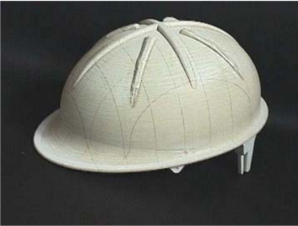
Figure 4: Rapid prototype pattern of hard hat in laminated paper
