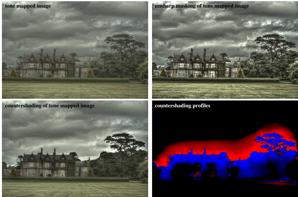
Figure 7: Image tone mapped using the contrast equalization [MMS06] (top/left) and restored by adaptive countershading (bottom/left). The restored image better communicates the brightness relations and the depth in the image. (top/right) shows unsharp masking with parameters set manually to equal dominant countershading profile. Although overall enhancement of unsharp masking is impressive, the changes are hardly controllable and modify the style of the image.
