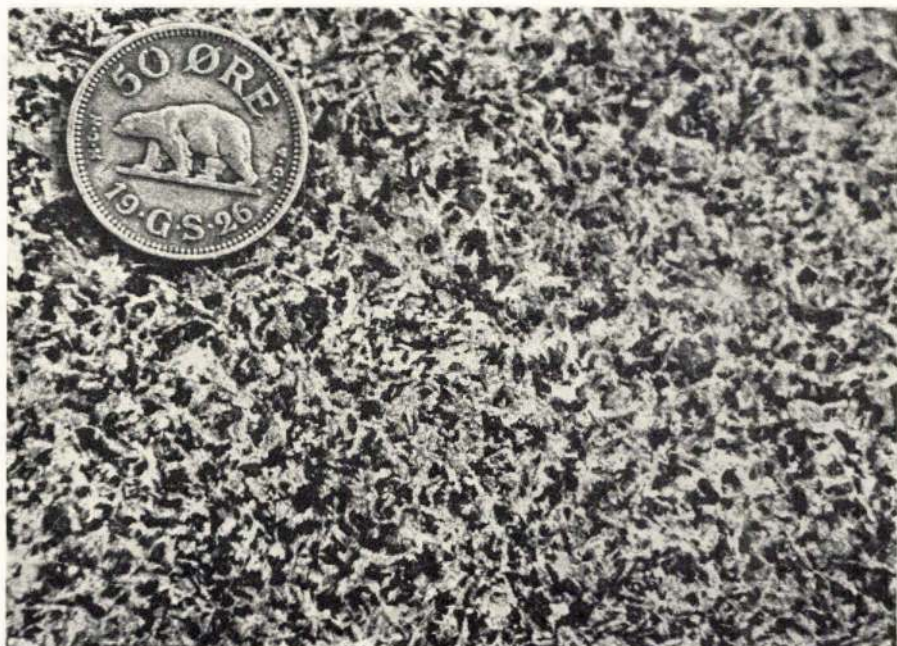
Fig. 13. Texture of metagabbro (3rd episode basic intrusion). The primary pyroxene has been partially replaced by hornblende but with the preservation of the ophitic texture. Diameter of the coin 2.2 cm. Photo: PREBEN CHRISTENSEN.
