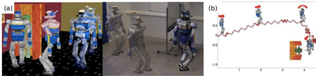
Figure 5.15: Extracted with author permission from [Sree09]. (a) HRP2 being maneuvered through space to find distant, hidden objects. (b) Plot of head position (solid line) and center of mass (CoM) position (dotted line) during motion. The zig-zag motion of the head and CoM position was due to the user alternatively looking left and right at every step.
