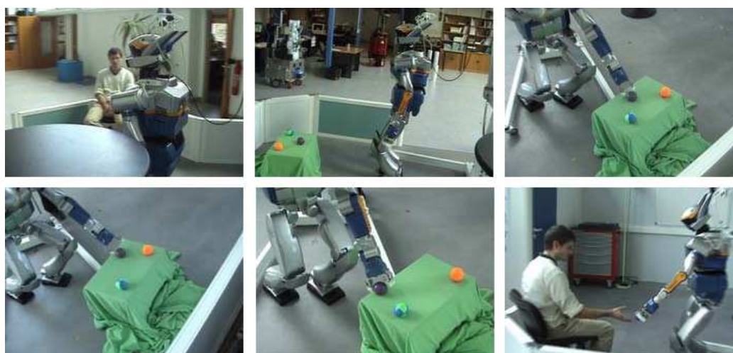
Figure 5.11: Second experiment instance. The robot is asked to give the purple ball to the person sitting on a chair. It walks toward the table, avoiding known obstacles in the environment. It first fails to grasp the ball (image 3 and 4), but with a simple error recovery strategy it finally succeeds (image 5) and accomplishes the mission.
