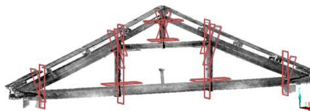
Fig. 5: Examined truss extracted from the Chorus point cloud. The red rectangles indicate the clipping boxes used for the sectioning of the cloud. Such clipping boxes measure 1 cm of thickness, which means they isolate the points contained in 1 cm, they are located in proximity of the knots between the elements and oriented perpendicularly to them.
