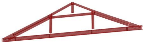
Fig. 10: Result of the modelling process; the algorithms implement the sweep of each section through the binary defined by the polyline connecting their barycenters.
