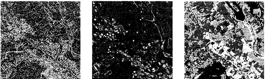
Figure 4. Extracts of texture and variance channels and of final land use map
