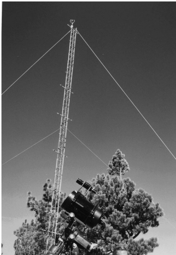
Fig. 1. The DIMM telescope (in front) and the instrumented mast during the May 2000 campaign.
