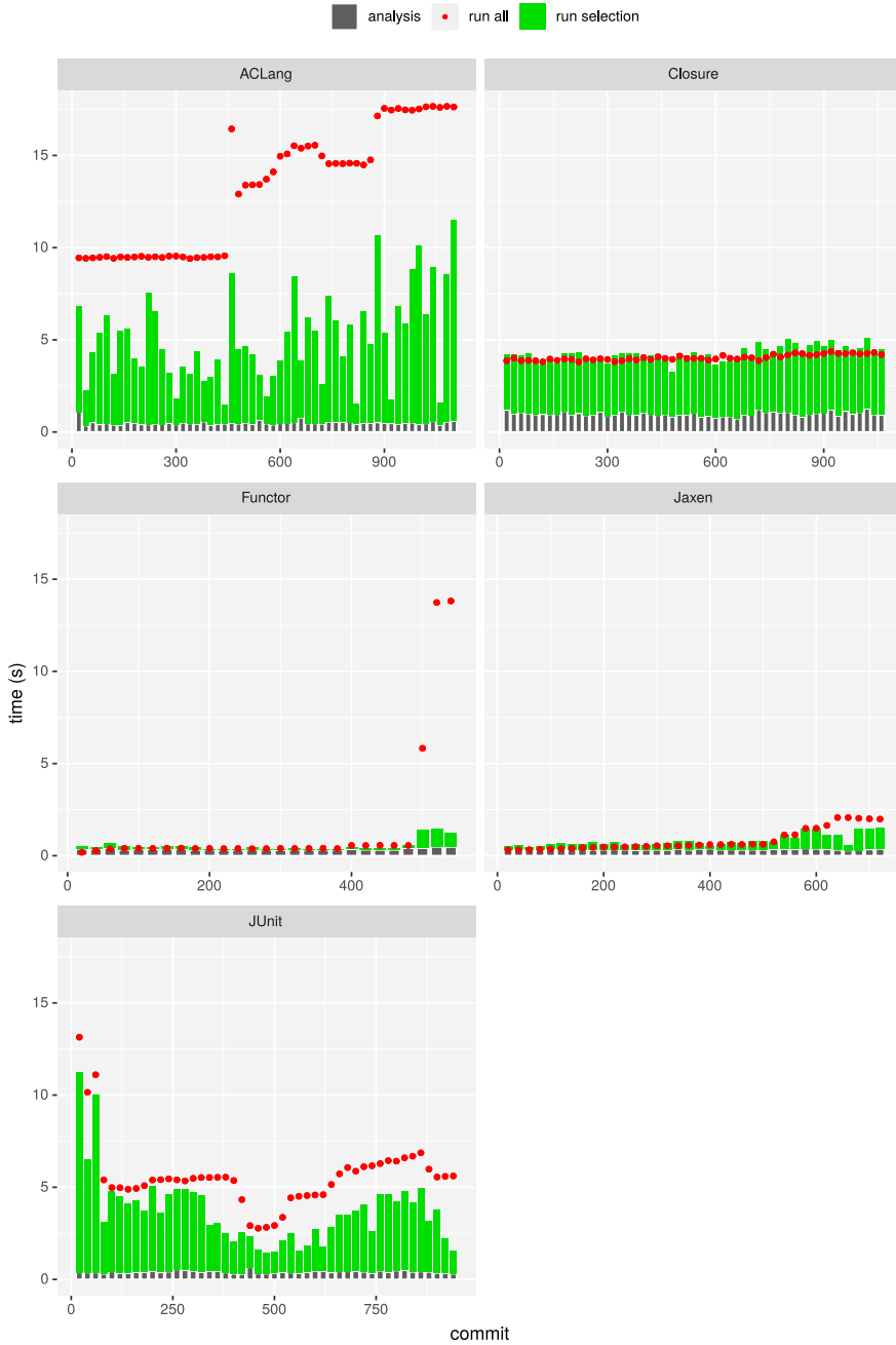
Figure 5: Testing time, means for bins of 20 commits. Test selection pays off when the red dot is above the stacked bars.
