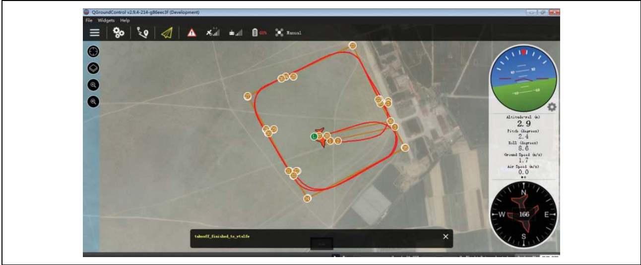
Figure 8. Flight trajectory and navigation points displayed in QGroundControl, the red line is actual trajectory, the orange is the designed trajectory.
