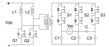
Figure 9. Series interfacing of active power APDC.
