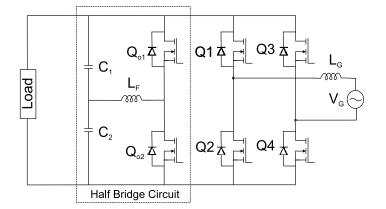
Figure 17. Half-bridge split capacitor proposed in [94].
