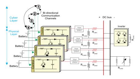
Figure 37. Virtual impedance control at nodes of microgrid.
