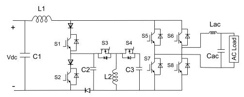
Figure 4. Active power filter for CSIs.
