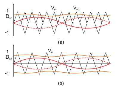
**Figure 30.** PWM strategy proposed in [130]. (a) Positive shoot through duty (in orange) with two triangular repeating waveforms (in black and dotted). (b) Positive and negative shoot through duty (in orange) with just one repeating singal (in black triangular), desired output sine wave is shown in red.
