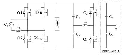
Figure 16. Symmetrical half-bridge configuration proposed in [93].
