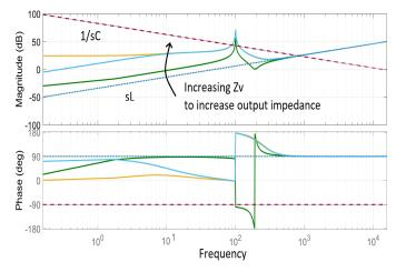
Figure 19. Variation output impedance with Zv.
