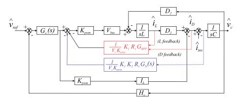
Figure 26. BPFICF with parallel impedance loop.
