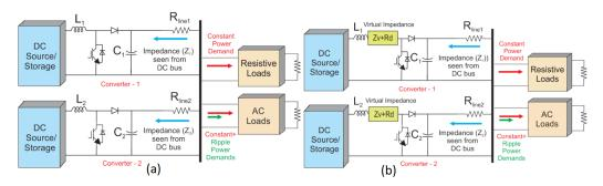
**Figure 1.** Impedance of node in microgrid (**a**) Without droop and virtual impedance Zv. (**b**) With droop Rd and Zv, if the  $Z_1 > Z_2$  ripple in node-2 will be more. This is regulated using Rd and Zv virtually.
