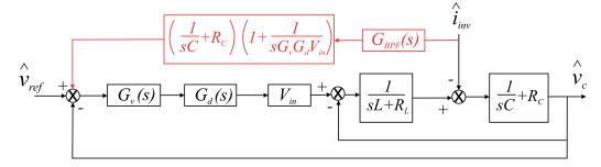
Figure 20. Load current feedforward methodology.
