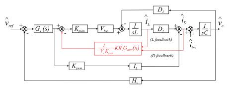
Figure 24. Bandpass filter inductor current feedback scheme.
