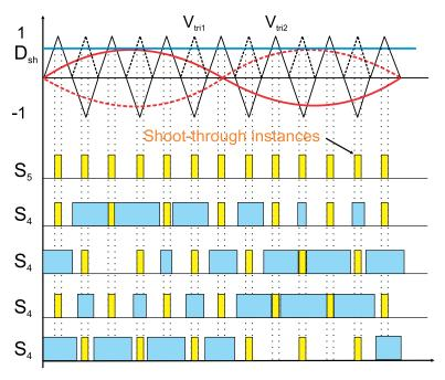
Figure 31. Conventional PWM for SSIs.
