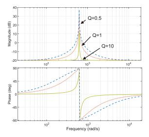
Figure 25. Notch characteristics with different Q-values.
