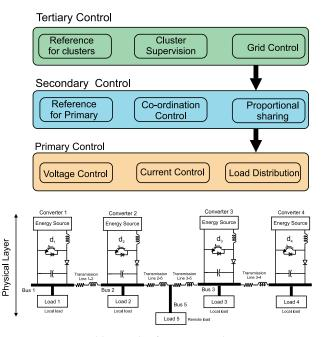
Figure 34. Control hierarchy for microgrids.
