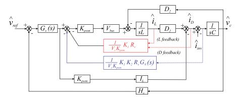
Figure 27. Notch-filter-inserted load current feedforward scheme (NF-LCFFS).
