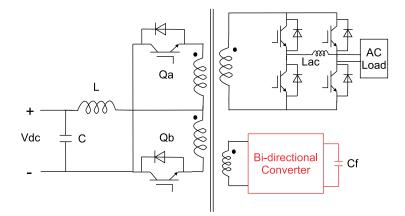
Figure 7. High-frequency flyback based utility interactive topology.
