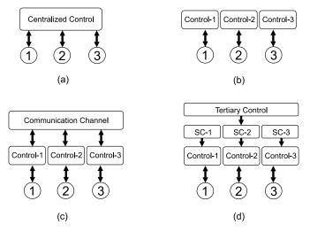
**Figure 33.** Concept of centralized and decentralized control: (**a**) Centralized control. (**b**) Decentralized individual control. (**c**) Distributed control with communication channel. (**d**) Multiple control levels as orimary, secondary control (sc), and tertiary controls.
