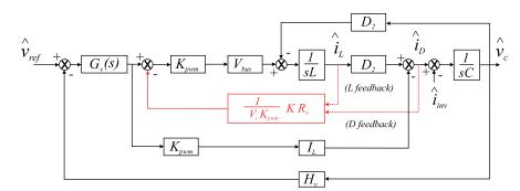
Figure 23. Virtual resistance scheme.
