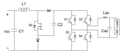
Figure 5. Active power buffer for CSI.
