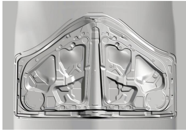
Fig. 5 Design of die addendum and binder surfaces of the part
