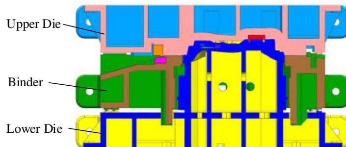
Fig.10 The upper and lower dies fully matched (the displacement of the upper die was 151.2 mm)
