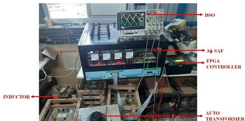
Figure 10. Experimental setup of DSTATCOM.
