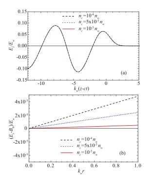
FIG. 1. Plasma wakefield excited by a quasi-matched, resonant Gaussian laser pulse with  $a_0 = 1$ and  $k_w w_0 = 2.3$  in a near-hollow plasma channel with  $k_w r_c = 1.5$  and  $n_c/n_w = 10^{-5}$ ,  $5 \times 10^{-5}$  and  $10^{-4}$ . (a) Accelerating wakefield  $E_z/E_w$  in the channel versus  $k_w(z - ct)$ . (b) Focusing wakefield  $(E_r - B_\theta)/E_w$  in the channel (at the peak  $E_z$ ) versus  $k_w r$ .
