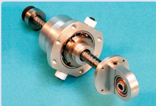
FIGURE C A prototype inerter. This translational inerter employs a ballscrew to convert the linear motion of the plunger into rotational motion of the flywheel (not shown). The device has a mass of approximately 1 kg and an inertance in the range 60–200 kg depending on the size of the flywheel. The device was designed by N.E. Houghton and manufactured in the Cambridge University Engineering Department.
