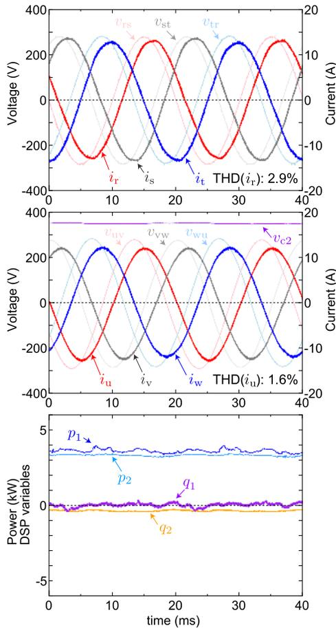
Fig. 13. Experimental waveforms for balanced resistive load. The primary side line currents,  $i_r$ ,  $i_s$ , and  $i_t$ , secondary side line currents,  $i_u$ ,  $i_v$ , and  $i_w$ , and capacitor voltage,  $v_{c2}$ , with the proposed control are shown. The variables used in the DSP, namely,  $p_2$ ,  $q_2$ ,  $p_1$ , and  $q_1$  are also shown.
