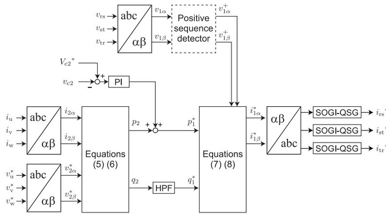
Fig. 4. Block diagram of proposed control for  $v_{c2}$ . It consists of feed-forwarding instantaneous power variables at the secondary side to the primary side current controller, and a simple PI feedback control.
