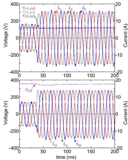
Fig. 19. Experimental waveforms for step change response. A balanced resistive load was applied in step, in addition to an additional balanced resistive load.
