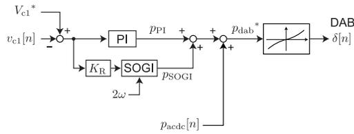
Fig. 2. Block diagram of proposed control for  $v_{c1}$ . It mainly consists of feed-forwarding power inflow from the AC side,  $p_{acdc}$ , to the dual active bridge (DAB) control, and a feedback control with a resonant controller. The latter is implemented using a SOGI.
