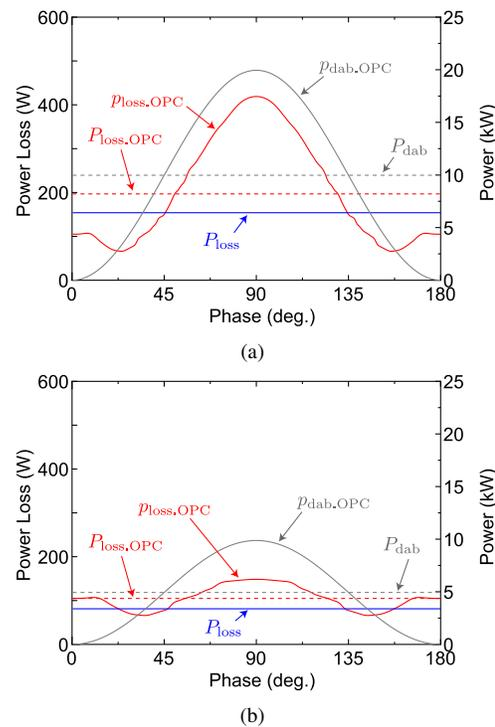
Fig. 24. Instantaneous power loss with the proposed OPC,  $p_{\text{loss.OPC}}$ , in a half line cycle, its average,  $P_{\text{loss.OPC}}$ , and loss with conventional control,  $P_{\text{loss}}$ , with (a) Rated power (9.97 kW) operation, and (b) 4.94 kW operation. The reference power for the OPC,  $p_{\text{dab.OPC}}$ , and its average (and therefore the reference power for the conventional control),  $P_{\text{dab}}$ , are also shown.
