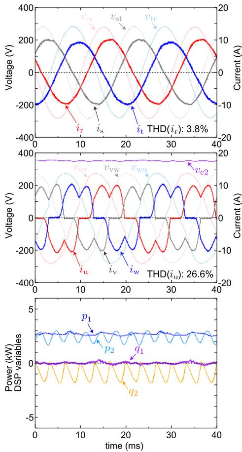
Fig. 17. Experimental waveforms for non-linear load with the proposed harmonic current compensation.
