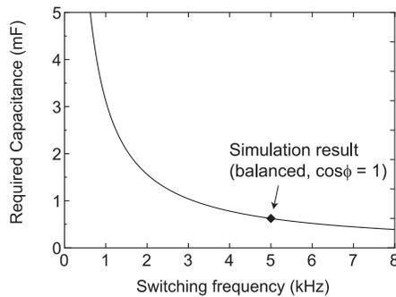
Fig. 8. Capacitance  $C_2$  required to achieve 5% voltage ripple with the proposed control albeit without harmonic compensation capability for the considered 300-kVA SST as a function of the switching frequency,  $f_{sw.dcac}$ .
