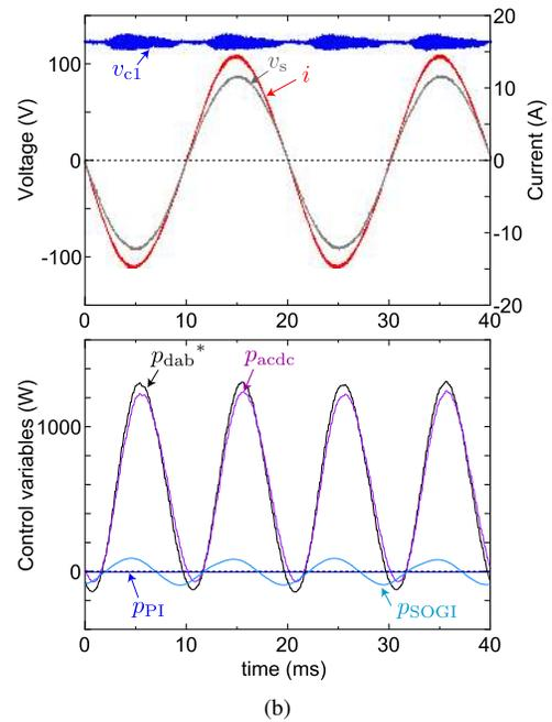
Fig. 11. Experimental waveforms and control variables in DSP with  $I_{rs} = 10$  A: (a) with conventional control and  $C_1 = 1600$   $\mu\text{F}$ , (b) with the proposed control, including feed-forward control and resonant controller tuned at 100 Hz and  $C_1 = 21.5$   $\mu\text{F}$ .
