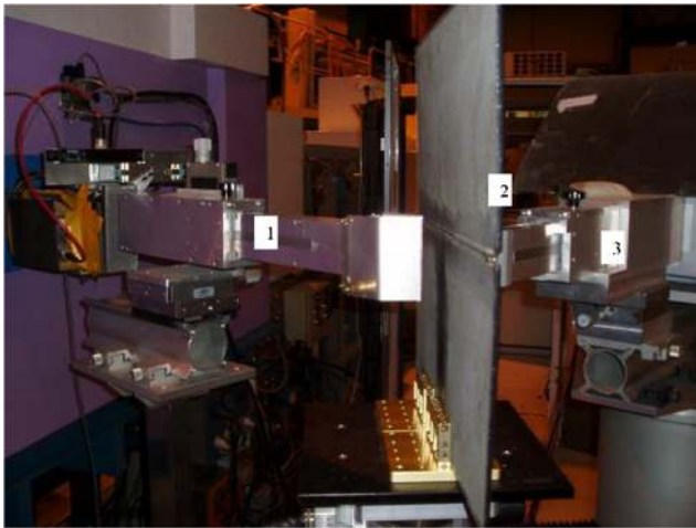
Fig. 5 Overview of the set-up for the neutron diffraction measurements at LBB. The numbers indicate neutron guide (1), the sample (2) and the collimator (3)
