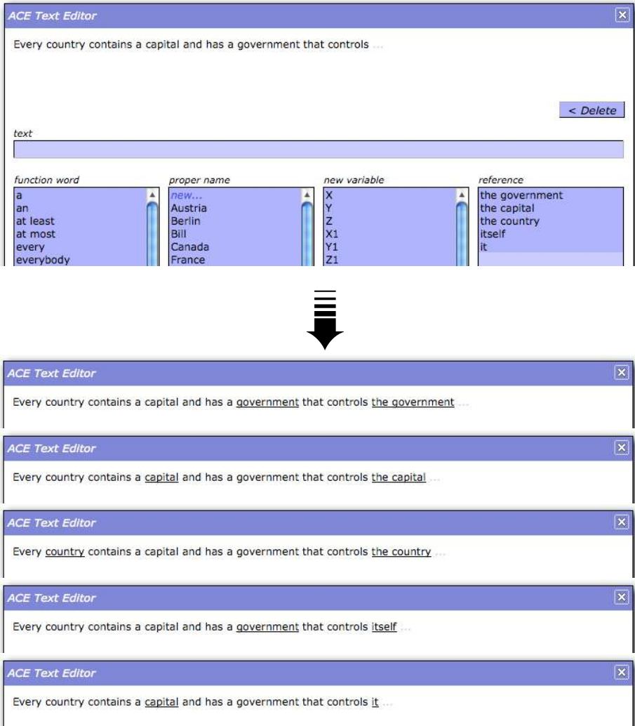
Figure 4.3: This figure shows how anaphoric references are handled in the predictive editor. At the top, the window of the predictive editor is shown with a partial sentence which can be continued by using an anaphoric reference. At the given position five different references are possible, which are shown in the rightmost menu box “reference”. When the user clicks on one of these reference entries then the editor shows how the reference has been resolved by underlining the respective part of the text.
