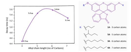
Figure 6. Decay times as function of alkyl chain length for derivatives A.
