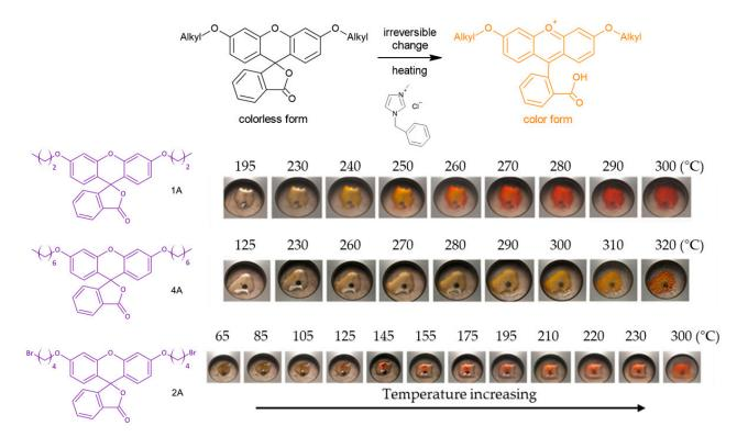
**Figure 7.** Scheme of thermochromic reaction of fluoran derivatives and IL (top) and changes of color during heating of fluoran derivative-IL mixtures.
