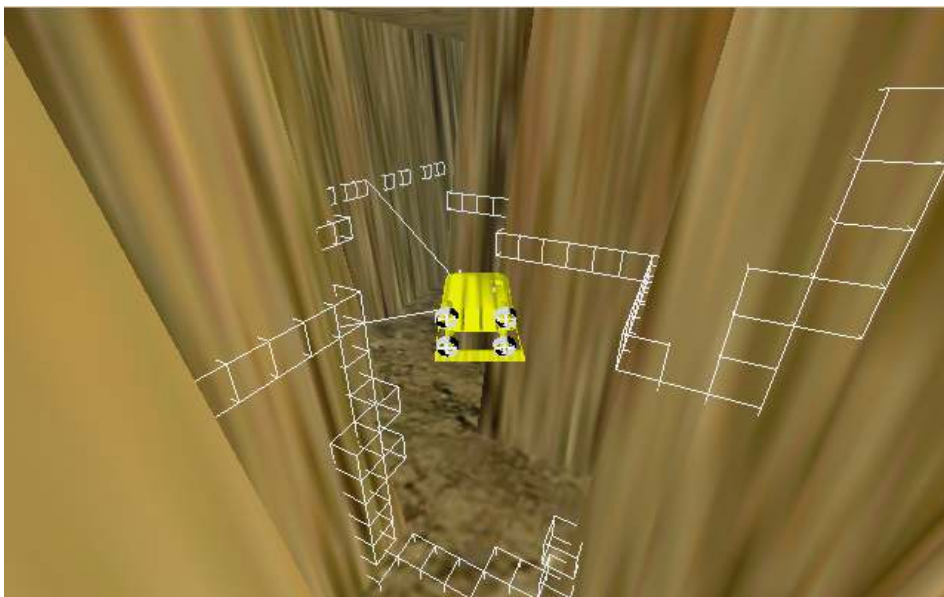
Figure B.1. The above figure shows a snapshot from the tunnel tracking test. The AUV should try to reach a way-point 700 m from the start position. The track has several turns and this figure illustrates one. Figure B.2 and B.3 illustrates the position and the utility functions at this specific time instance.
