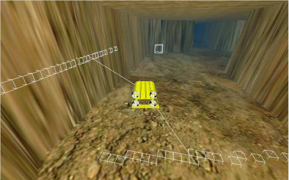
Figure 3.2. The following figure illustrates the simulator environment where two sonars have been added to the AUV. The first sonar is sweeping in the horizontal plane and the other in the vertical plane. The sonars are based on echo signals and the outputs are a range and a bearing to an obstacle. The white boxes illustrate obstacles, hit by the sonars. As can be seen in the figure the AUV is in a tunnel environment that also has been developed during the thesis.
