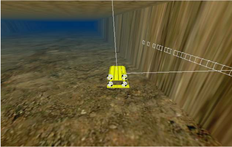
Figure 4.1. The above figure shows a snapshot from the wall tracking test. The AUV should try to reach a way-point behind a wall 300 m away from the start position. Two different tests are made for the comparison between the various heading spreads and control modes.
