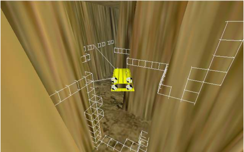
Figure 4.4. The above figure shows a snapshot from the tunnel tracking test. The AUV should try to reach a way-point 700 m from the start position. The track has several turns and this figure illustrates one.
