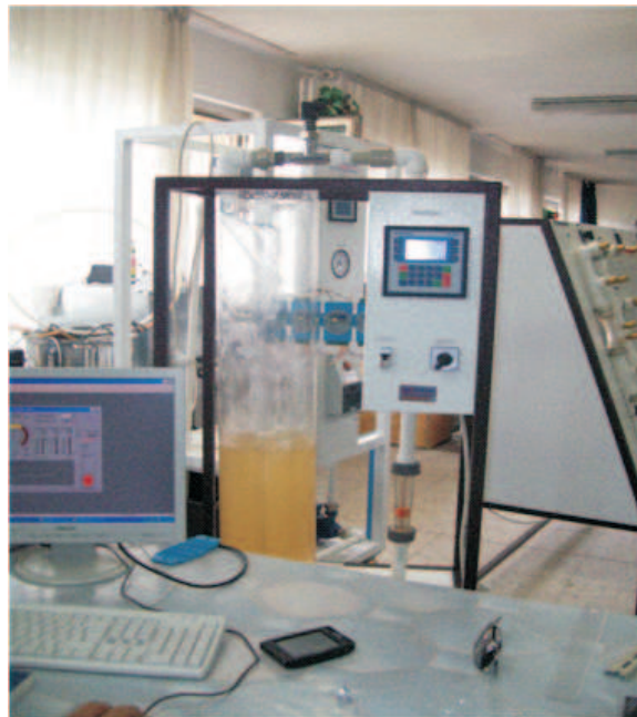
Fig. 2. Photo of water-level measurement device
