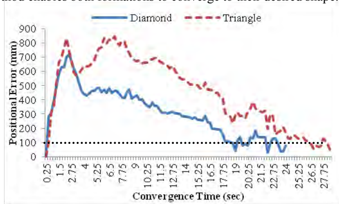
Fig. 7 Difference between desired and actual positions for followers as velocity of ML increased
