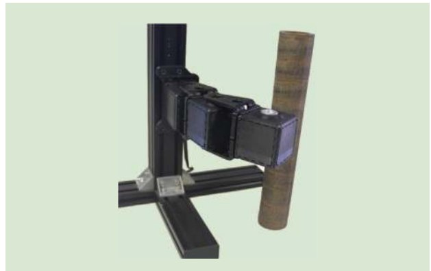
Figure 5. The experimental setup: a two-degrees of freedom (DoF) horizontal VSA arm built using Qbmove Maker Pro servo motors and a bar as an environmental constraint.
