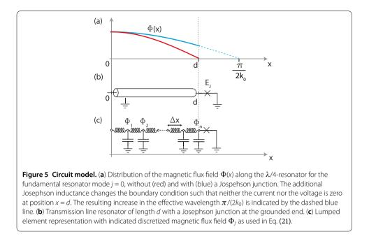
The total Lagrangian of the system in the magnetic flux field  $\Phi(x)$  has a transmission line part and a term which describes the SQUID at position x = d (Figure 5).
