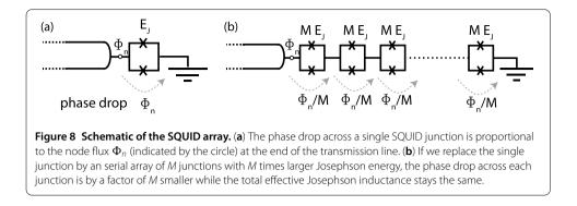
phase drop  $\Phi_n/M$  across each SQUID, see Figure 8. As a result the quadratic term in the Lagrangian scales as
