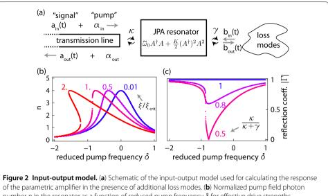
number *n* in the resonator as a function of reduced pump frequency  $\delta$  for effective drive strengths  $\xi/\xi_{crit} = 0.01, 0.5, 1, 2$ , where  $\xi_{crit} = -1/\sqrt{27}$ . (c) Absolute value of the reflection coefficient  $|\Gamma|$  for different coupling ratios  $\kappa/(\kappa + \gamma) = 1, 0.8, 0.5$ .
