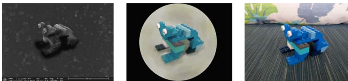
12 13 Fig. 1. Illustrating the challenge to synthesise a macroscopic object ( e.g. toy frog, right ) with the 14 same morphology at the mesoscale (light microscope image, middle ) and at the nanoscale (scanning 15 electron microscopy image, left ).
