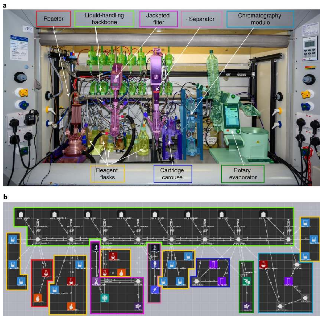
Figure 5: Implementation and topology of the synthesis platform. a, Physical instance of the Chemputer used for the synthesis of NHS-diazirine. The discrete modules are highlighted in different colours and labelled. b, Representation of the same instance in graph format; the modules are highlighted according to the colour code used in a.
