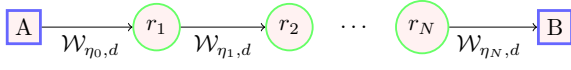
FIG. 6. Alice (A) and Bob (B) are connected by N quantum repeaters r_1, \dots, r_N in a linear chain; each connection (edge) in the chain is a d dimension HW channel with a generally-different parameter \eta_i .
