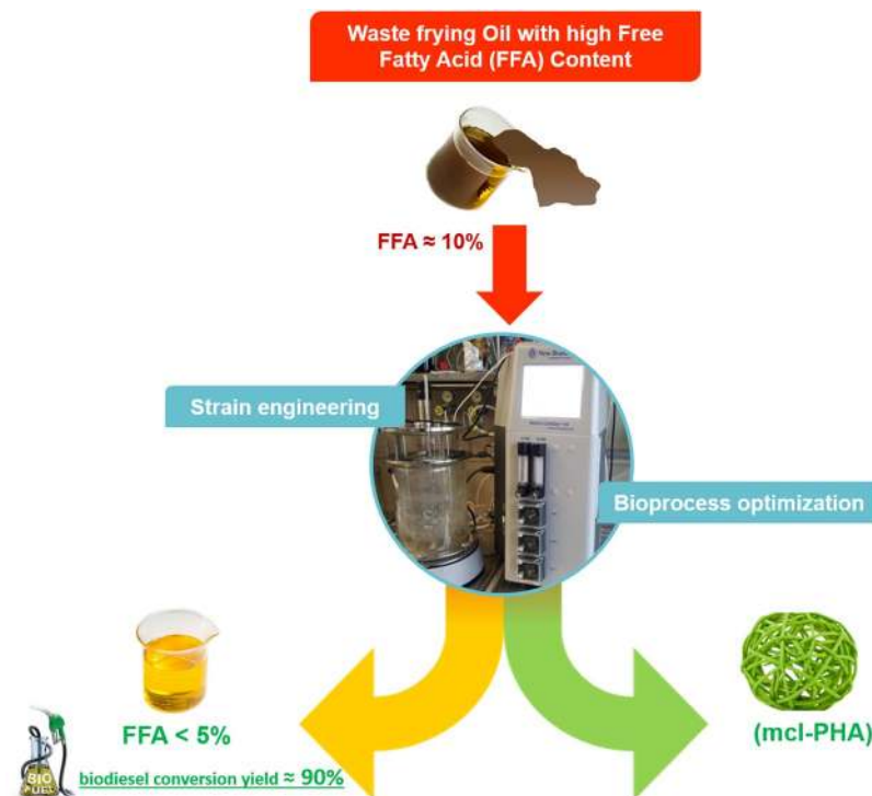
Figure 3. Schematic representation of the proposed multi-product process for the conversion of no/low value WFOs into biodiesel and biopolymers.
