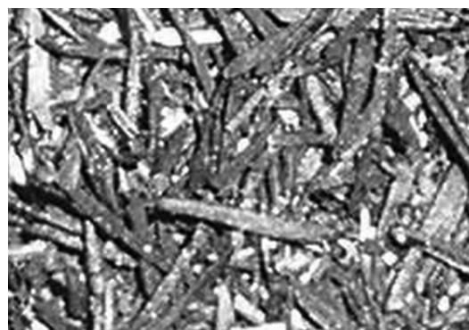
Figure 2. Macroscopy of RHA as received.
