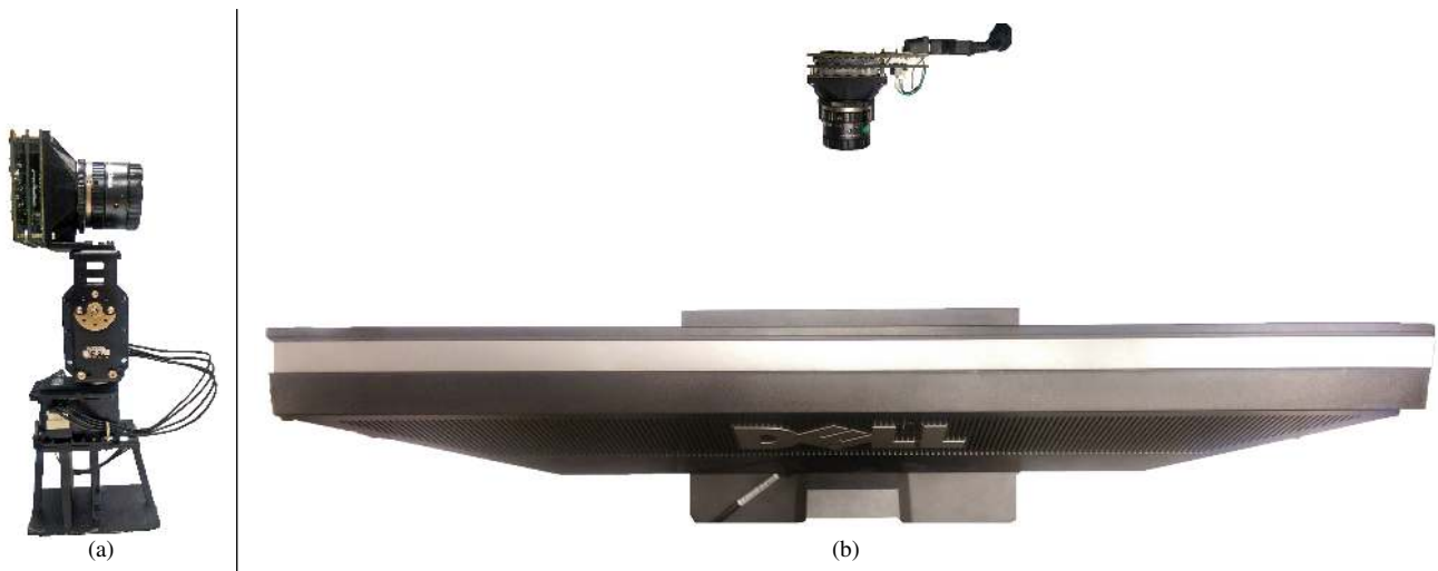
Figure 2. (a) A picture of the ATIS mounted on the pan tilt unit used in the conversion system. (b) The ATIS placed viewing the LCD monitor.
