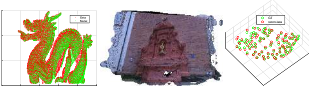
Figure 1: Non-minimal results obtained using our framework. From left to right: rigid registration (model: green; data: red) on the public dataset [15]; 3D reconstruction of the Fountain sequence obtained using the estimated camera intrinsics; non-rigid 3D reconstruction (ground truth: green; reconstruction: red) of tshirt with Lasserre’s relaxation.
