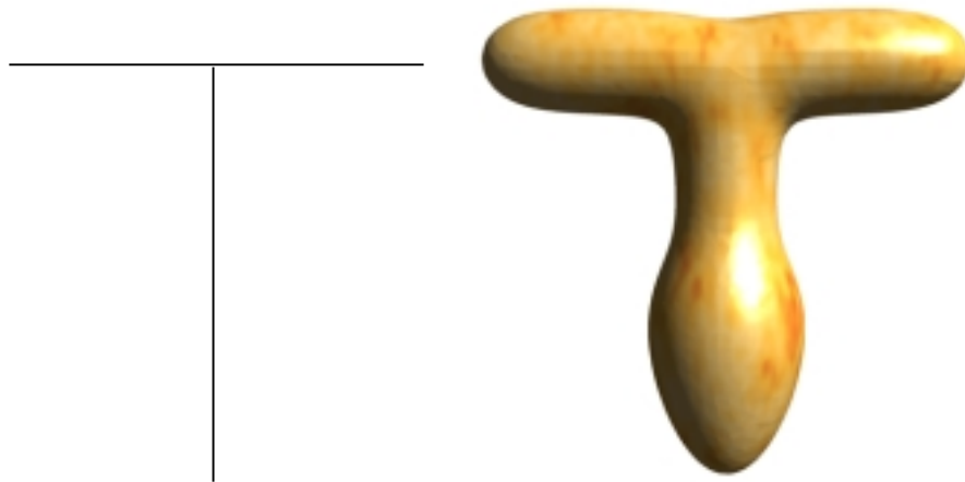
Figure 4. T-shape object. (a) Skeleton. (b) Convolution surface.
